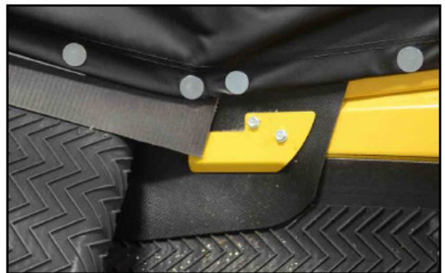
Fig 14 - Fasten flashing clamp
