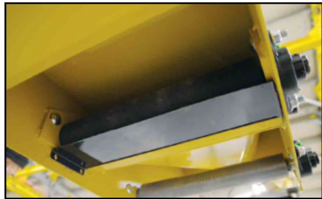
Fig 4 - Containment plate in place
