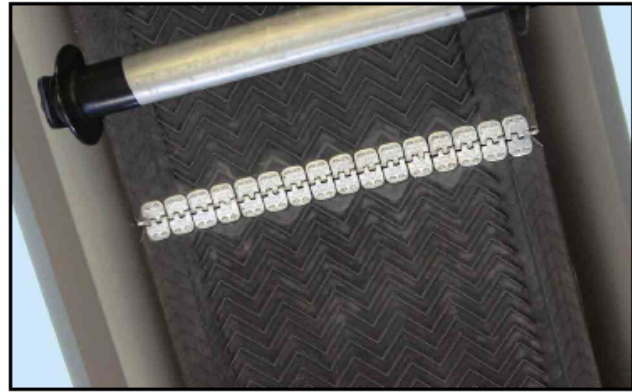
Fig 1 - Conveyor belt lacing
