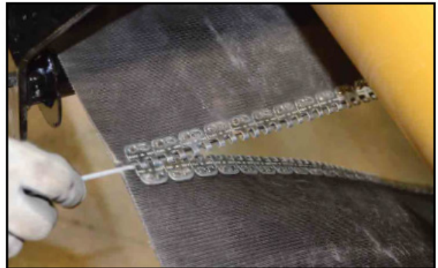
Fig 7 - Thread lacing cable
