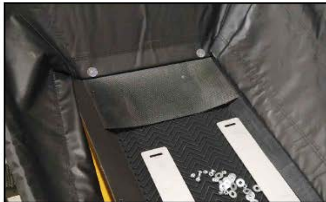
Fig 10 - Tail flashing on top of side flashing
