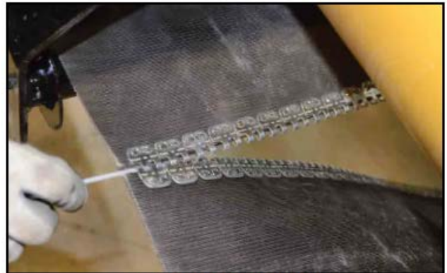
Fig 7 - Thread lacing cable
