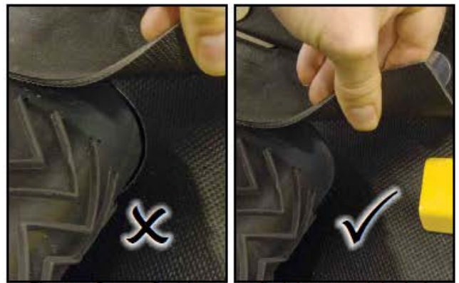
Fig 13 - Corner flashing must fit tight around the belt
