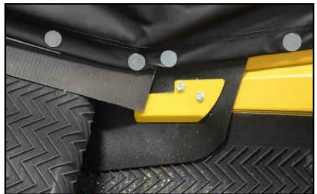
Fig 14 - Fasten flashing clamp
