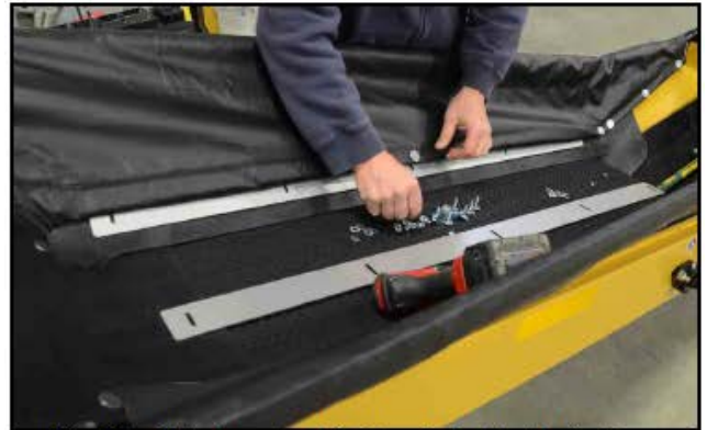
Fig 12 - Stainless steel flat bar to hold side flashing
