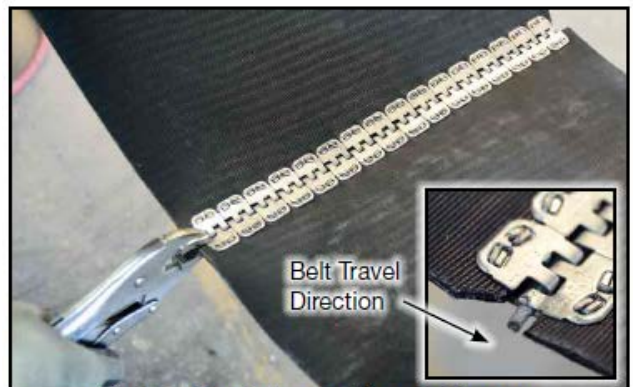
Fig 8 - Crimp lacing and taper belt corner
