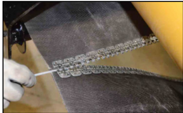
Fig 7 - Thread lacing cable
