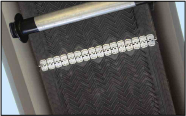
Fig 1 - Conveyor belt lacing
