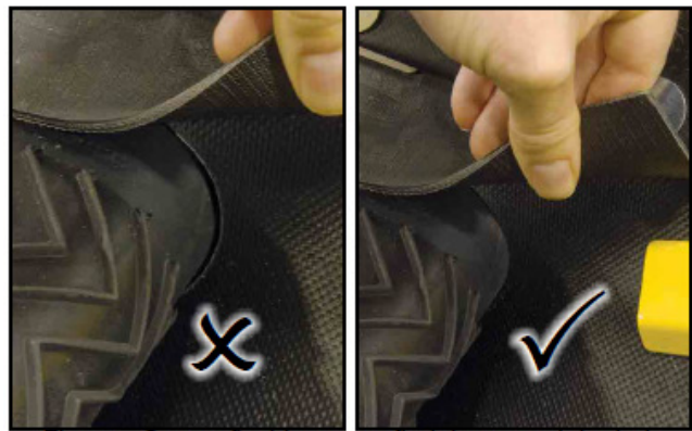
Fig 13 - Corner flashing must fit tight around the belt
