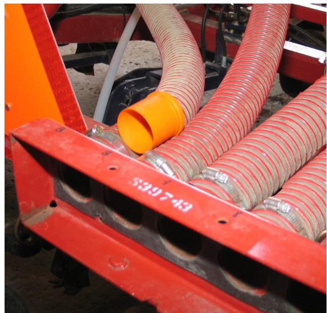
Insert Equalizers on Coupler Seeding Tool side
