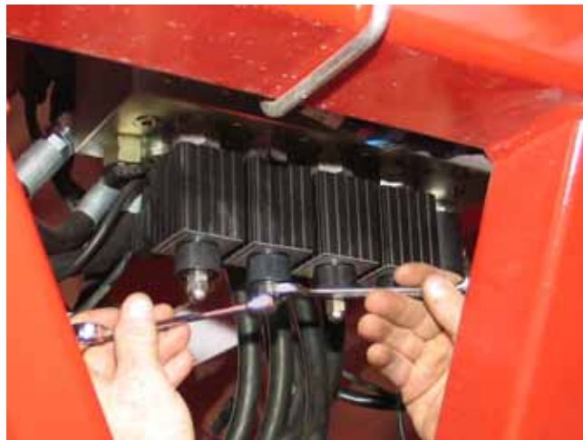
Remove Cap Nut and Loosen Jam Nut
