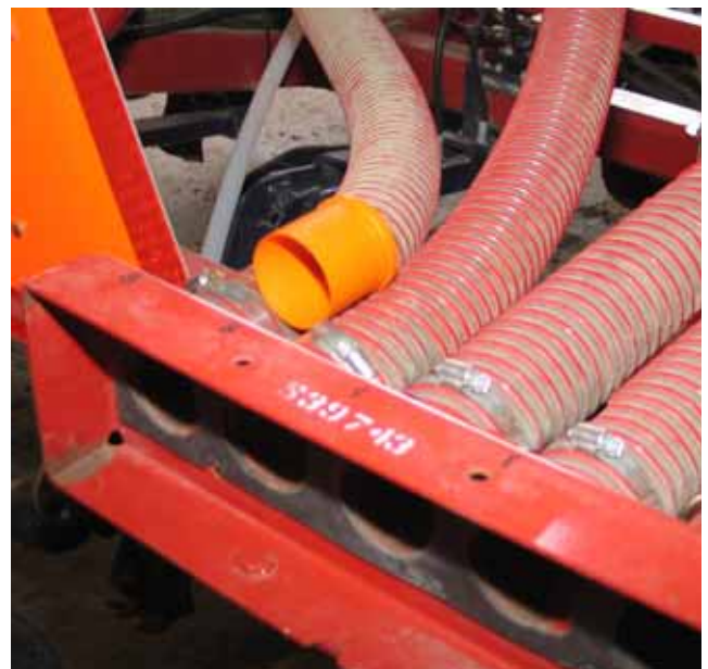
Insert Equalizers on Coupler Seeding Tool side
