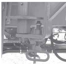
Auger Arm Lock Pin - Unlocked -
