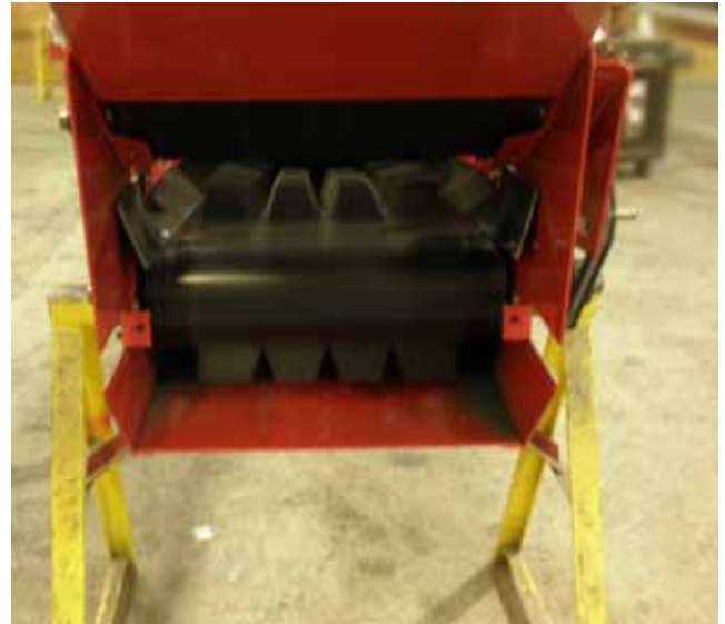
Open tail and center belt on rollers
