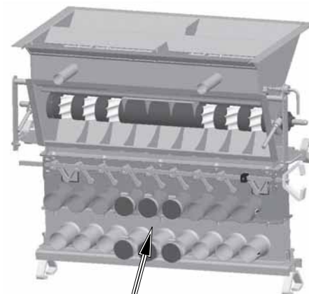
COLLECTOR Collector Valve Shown on "Bottom Pipe" Setting
