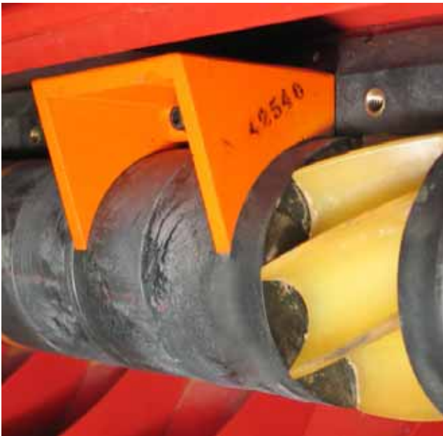
Correctly Installed Blank Off
