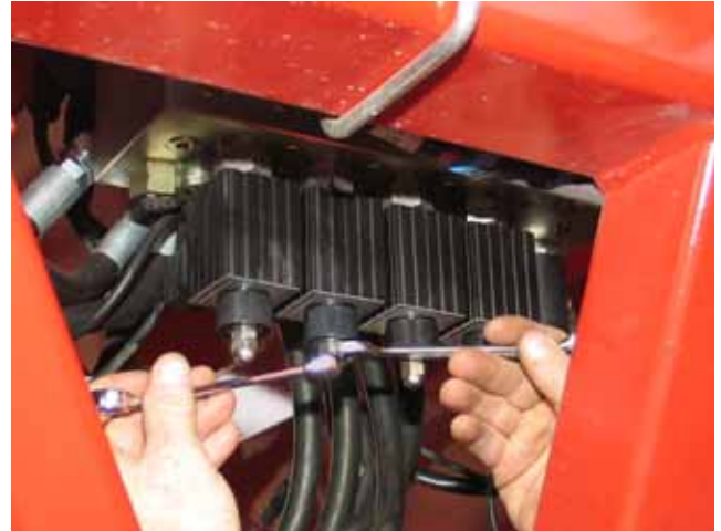
Remove Cap Nut and Loosen Jam Nut
