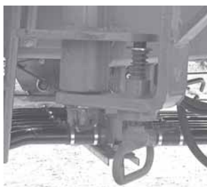
Auger Arm Lock Pin - Locked -
