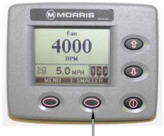
Pressing soft key under SMALLER will switch the screen back to the two - display sections.
