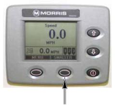
Pressing soft key under "Smaller" will switch the screen to the 2 - display sections.
