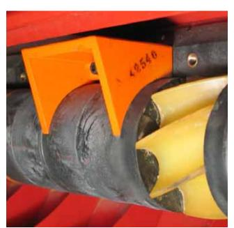
**Correctly Installed Blank Off**
