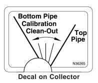
IMPORTANT **Cycle Collector Valve Daily** to ensure free movement. Minimum of 5 cycles.
