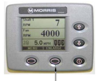
Press soft key under ENLARGE to enlarge bottom section.
