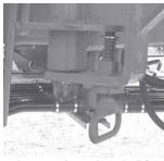
Auger Arm Lock Pin - Locked -
