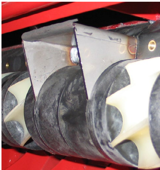
Correctly Installed blank-off
