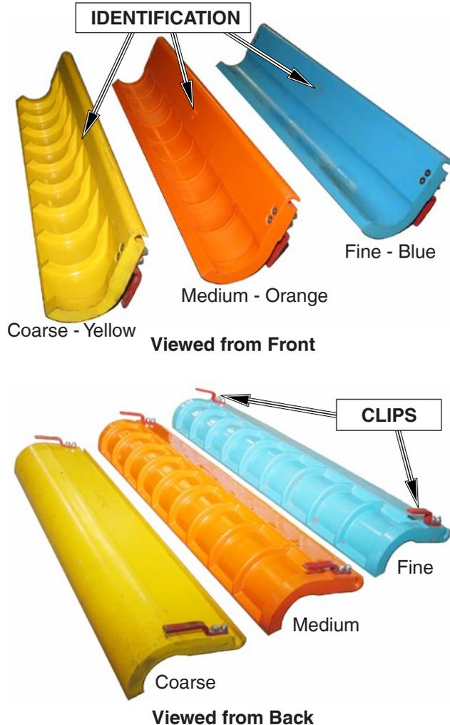
Seed Plate Assembly complete with clips:
