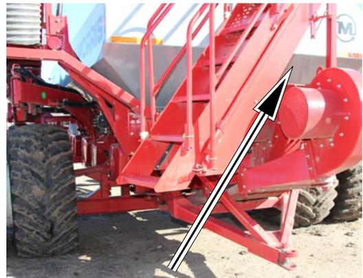
**Note:** Do not attempt to meter product when fan is not running. Damage to the metering wheels may occur.
