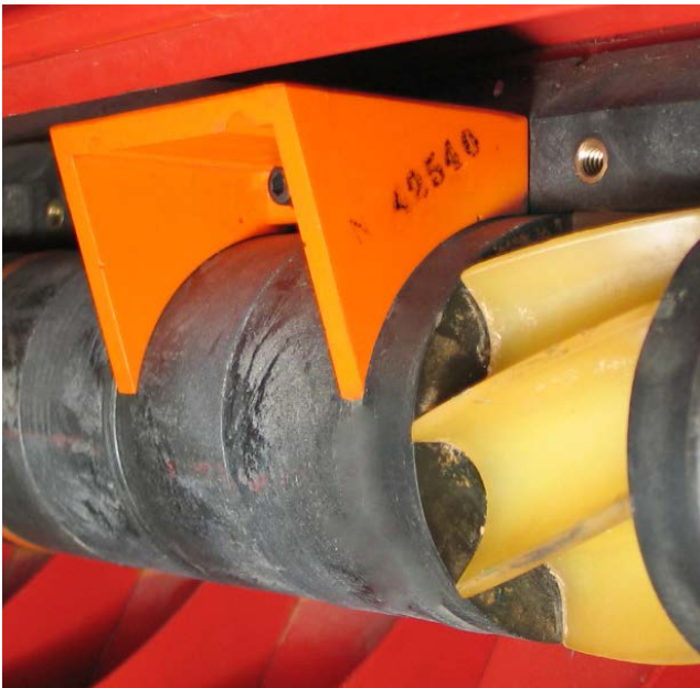
Correctly Installed Blank Off
