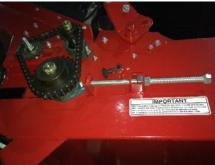
bolt in 2-3 turn increments. Run the conveyor after each adjustment to see the result.
