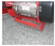
Access cover for incline conveyor cleanout
