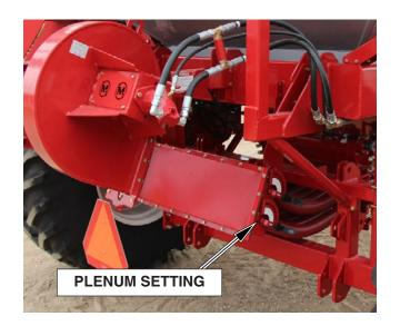
Set Plenum Damper so that setting is in the middle of slot.
