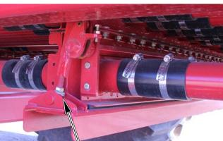
Adjust the latch bolts to obtain a force of 30 lbs (14 kg) to close the Door.
