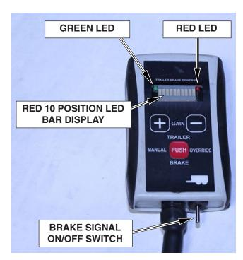
GREEN LED is ON when 12v power is in control.
