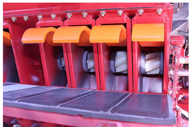
Inspect Metering Body
