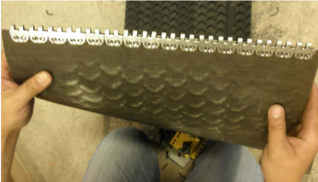
Bend fastener strips
