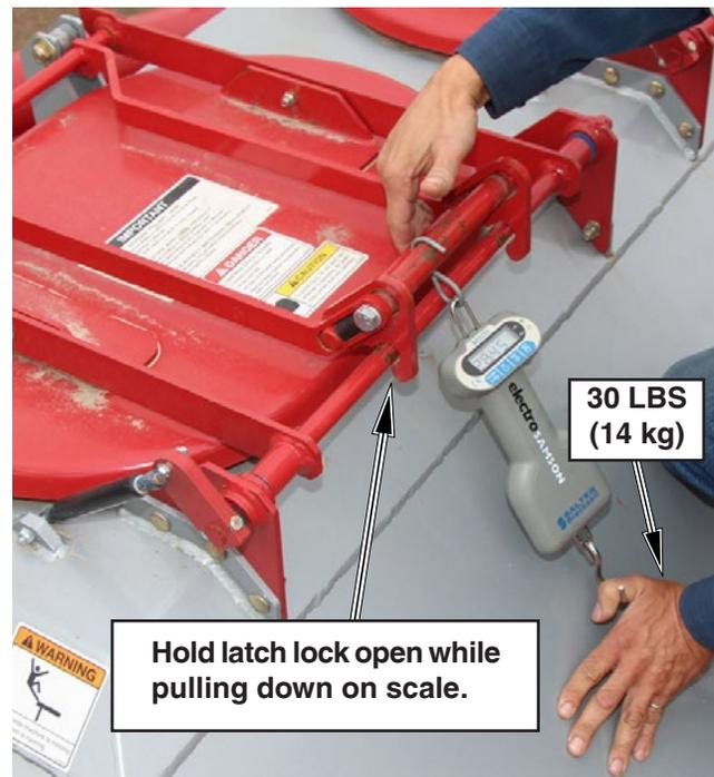
Adjust the lid latch bolts to obtain a force of 30 lbs (14 kg) to close the lid.
