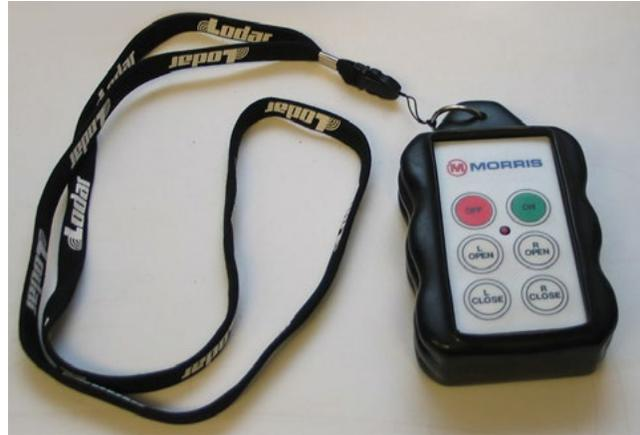
Meter Shut-Off Remote Control
