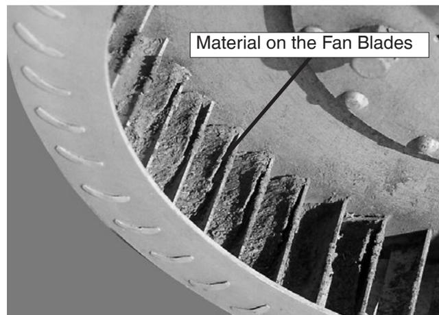
**Note:** Material build up on the fan blades could cause the fan to be out of balance. The added vibration of the out of balance impeller will reduce the life of the fan components.
