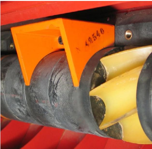
Correctly Installed Blank Off
