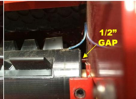
7. If adjustment is necessary, **TIGHTEN** the roller on the side of the housing that the belt is closest to, or rubbing on. Adjust bolt in 2-3 turn increments. Run the conveyor after each adjustment to see the result.
