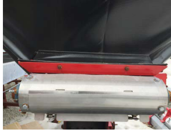
Access cover and door for hopper clean-out
