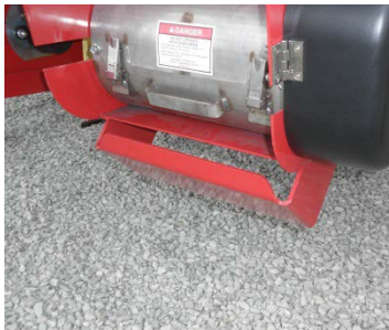
Access cover for incline conveyor cleanout
