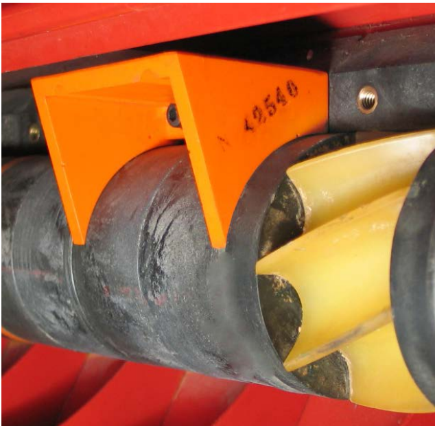
Correctly Installed Blank Off
