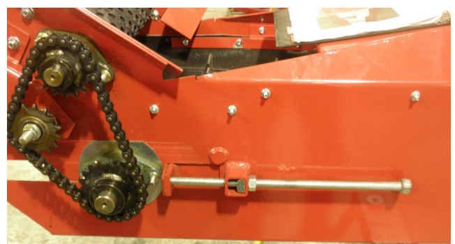
Right tensioning bolt
