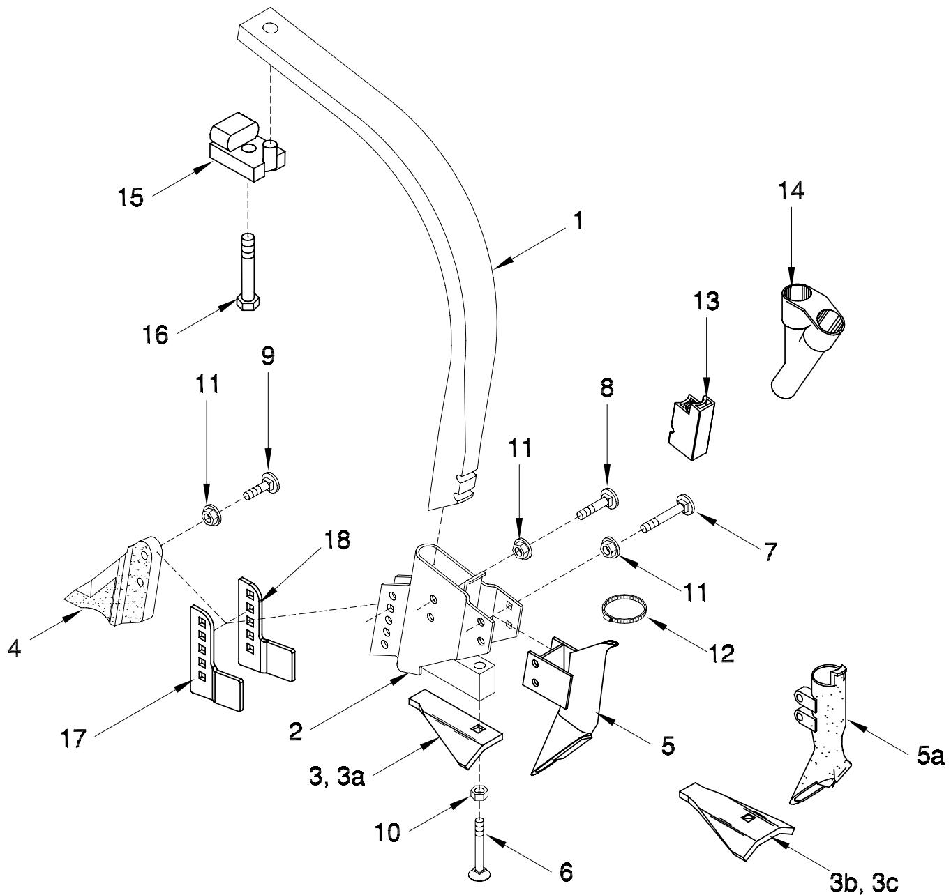
Note: Item 15 & 16 required on trips located behind transport wheels of the Maxim Air Drill.
