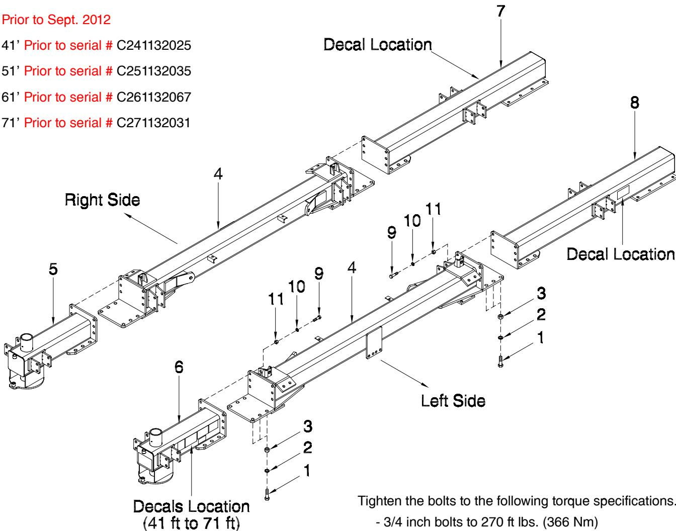
Tighten the bolts to the following torque specifications.
