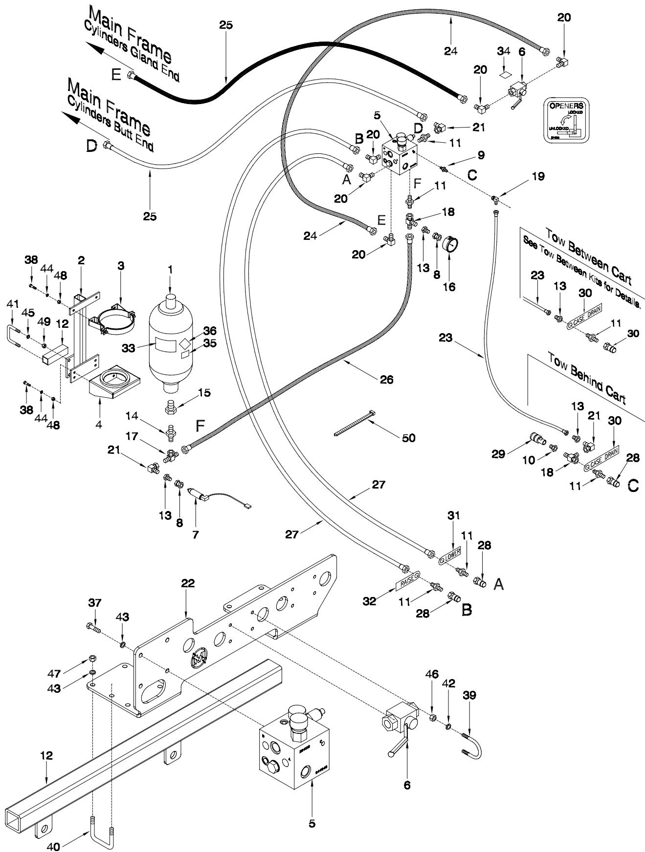
**Opener Hydraulics - 25 & 31 Ft Accumulator and Hitch Hydraulics - Prior to 2016**
