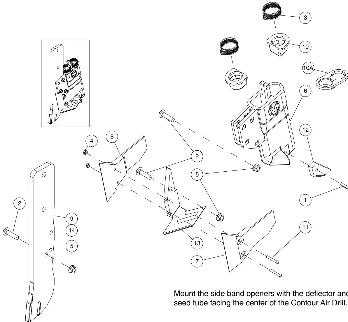
Mount the side band openers with the deflector and seed tube facing the center of the Contour Air Drill.
