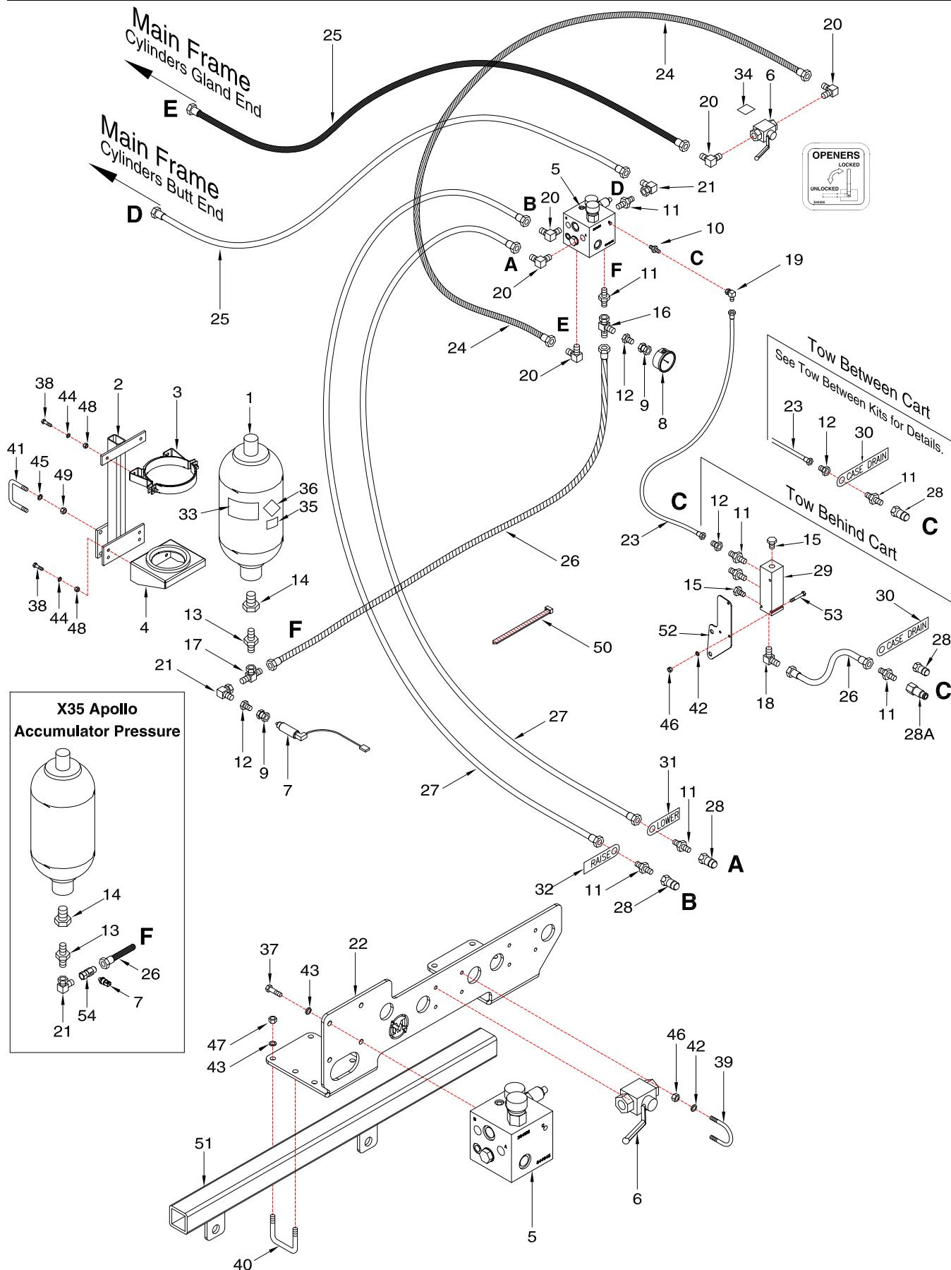
**Opener Hydraulics - 25 & 31 Ft Accumulator and Hitch Hydraulics - 2016 to Present**
