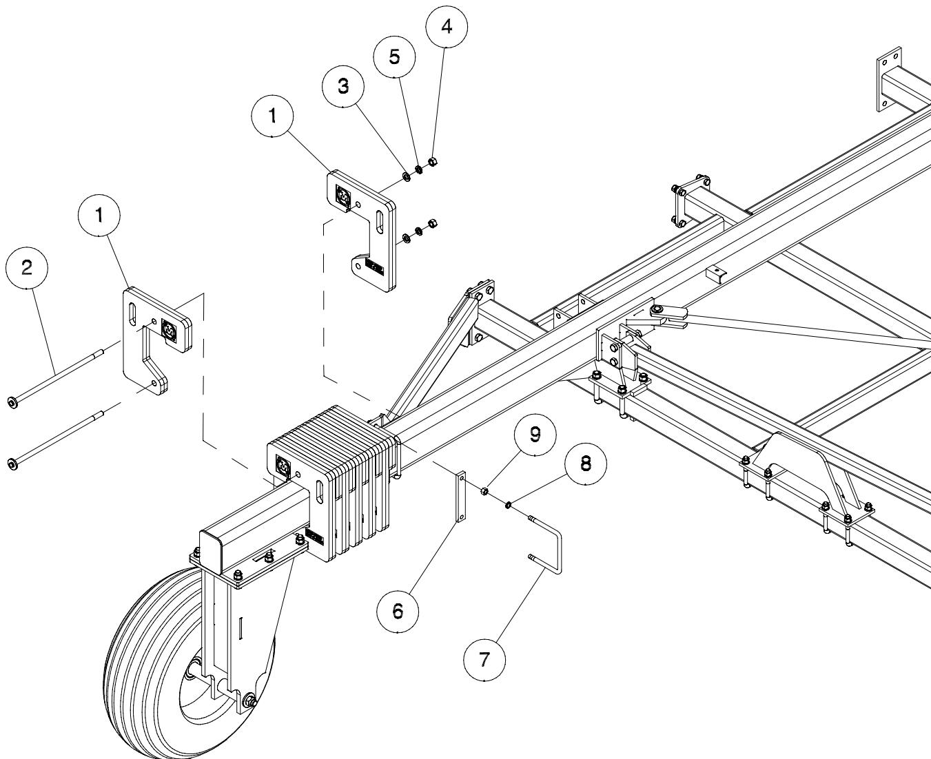
**Note:** Wrap Wieghts (1) around beam alternating left to right.
