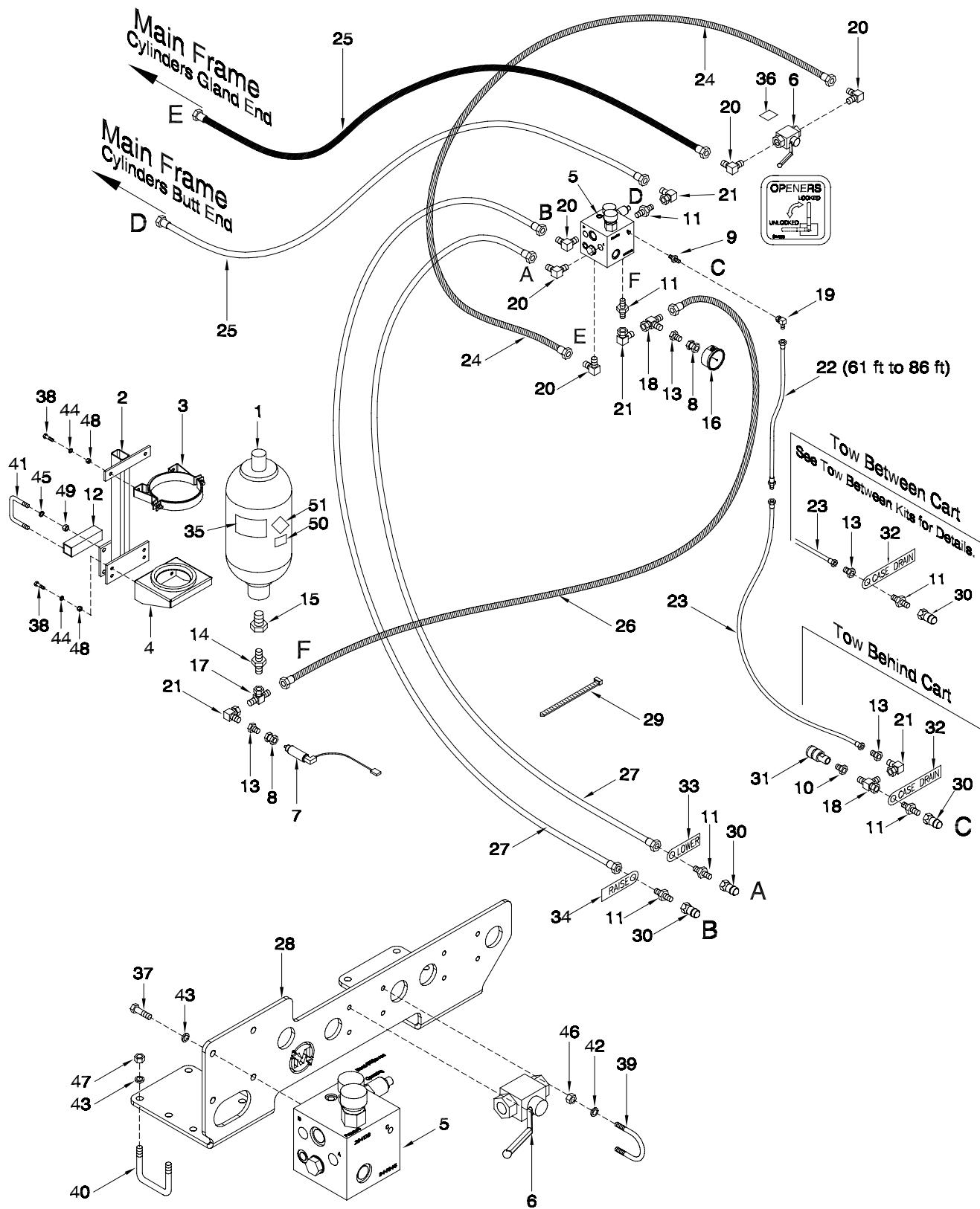
**Note:** Case Drain Tee with Quick Coupler must be moved to the front of a Tow Between Air Cart.
