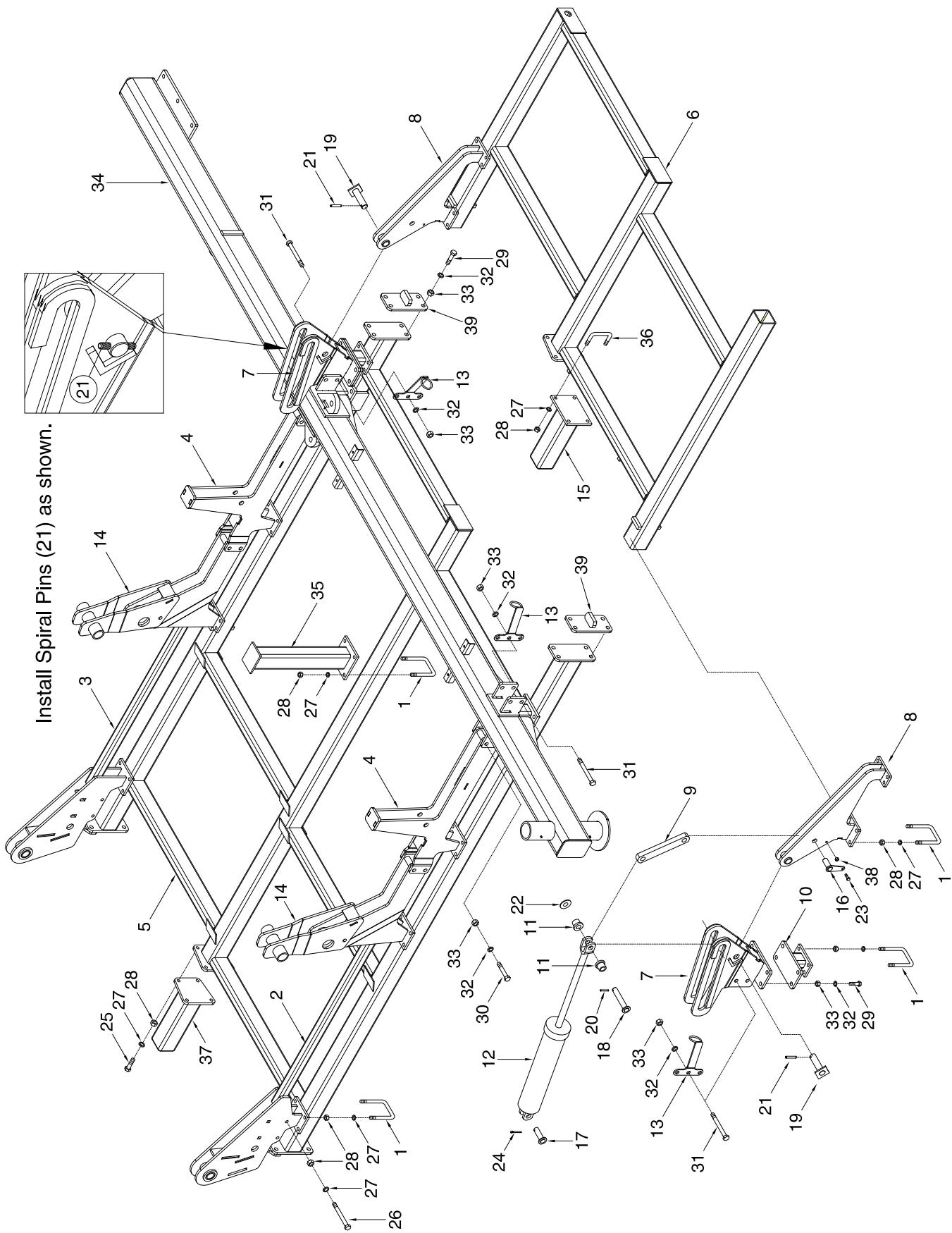
Install Spiral Pins (21) as shown.
