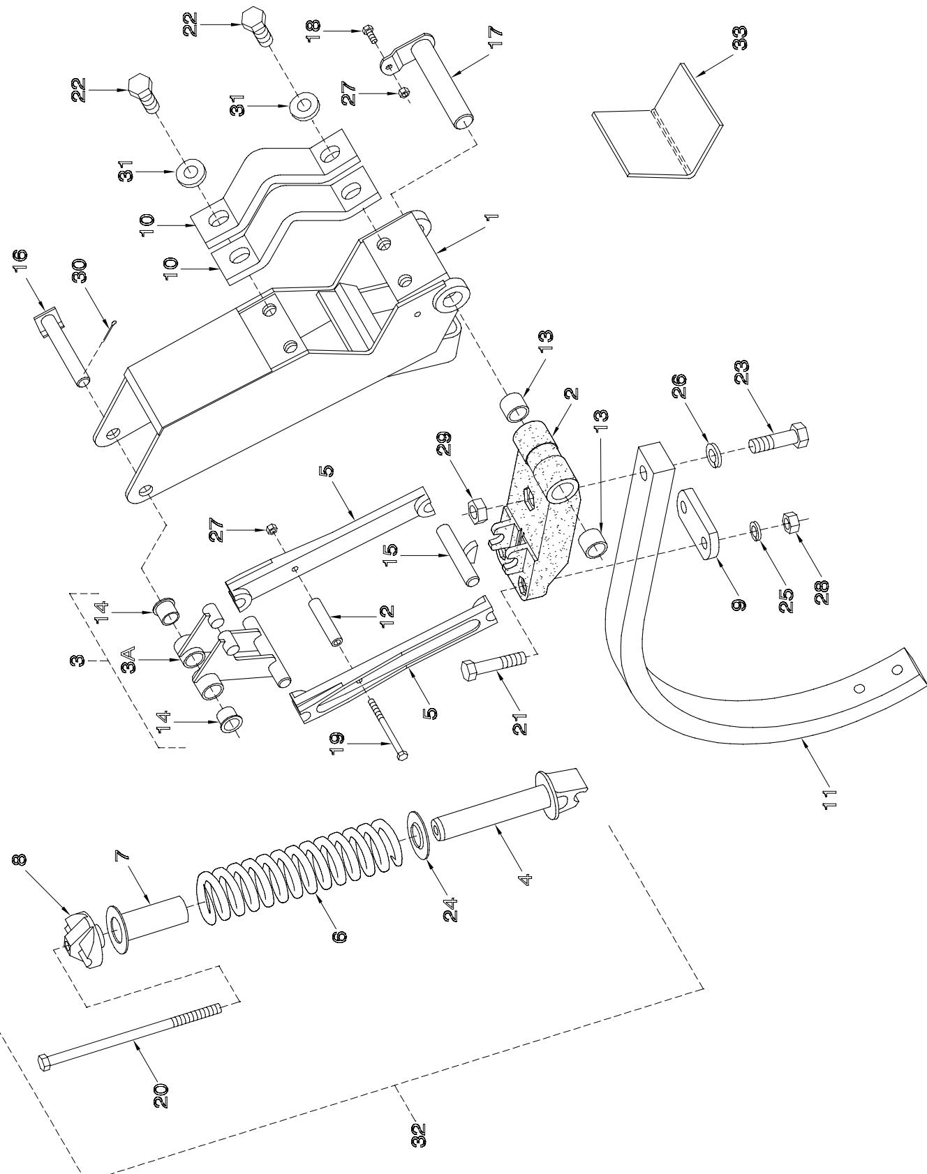
**Trip Assembly - LH 755 Trip - Spring 1998 to Spring 2002**
