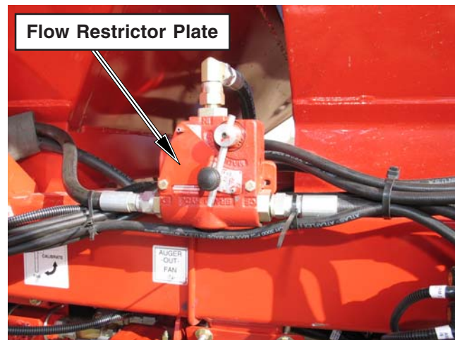
Flow Control Valve
