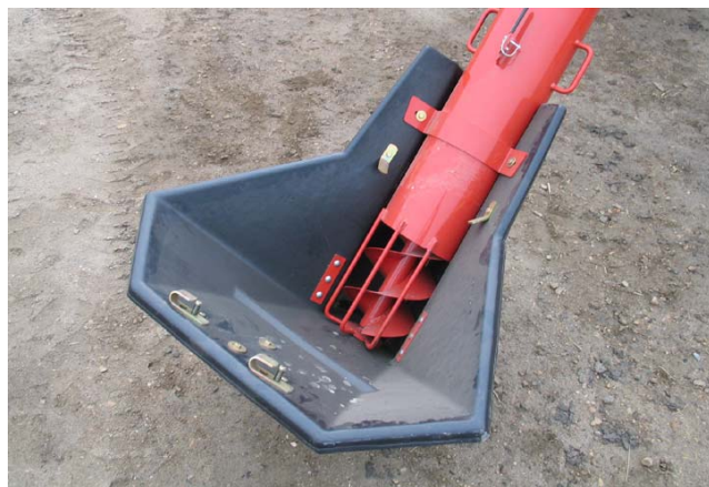
Auger screen removed
