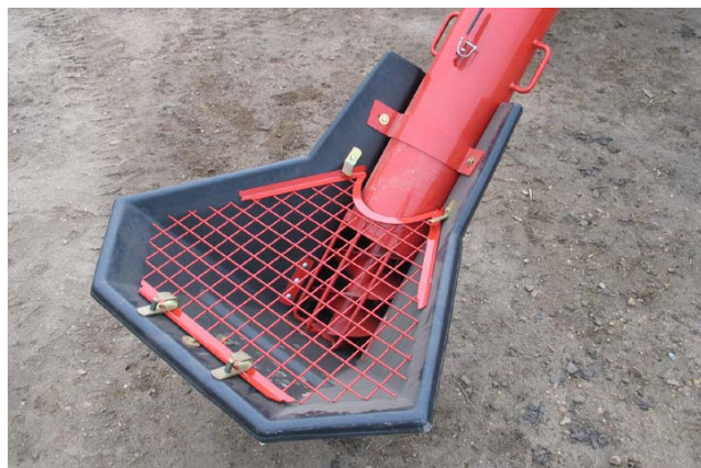
Auger screen installed
