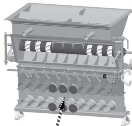
Collector Valve Shown on "Bottom Pipe" Setting
