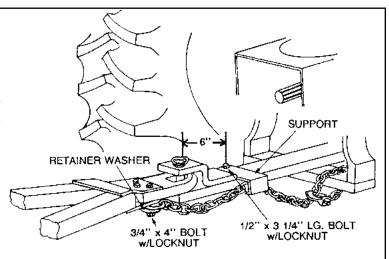
Attach safety chain to the tractor drawbar support or other specified anchor location with the appropriate parts.
