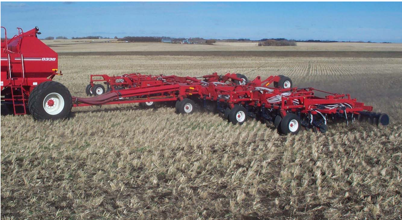
Shown: 60 foot Maxim III Air Drill on 10 inch spacing with 8336 VRT Air Cart
