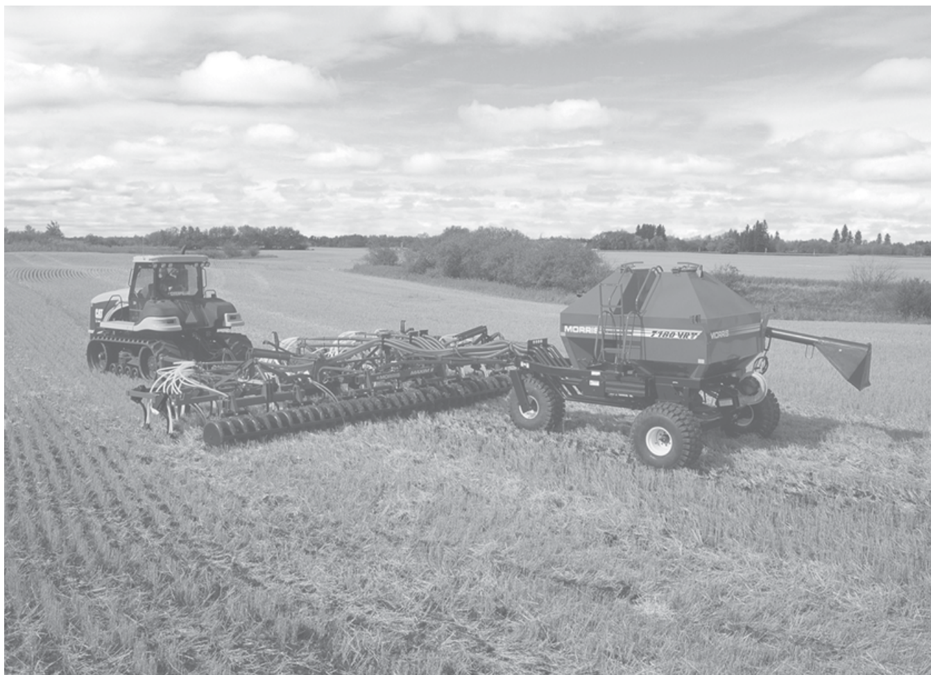
Shown: 34 foot Maxim II Air Drill on 10 inch spacing with 7180 VRT Air Cart
