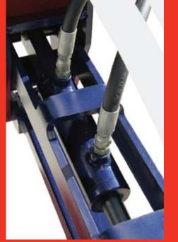
A double acting hydraulic cylinder raises and lowers the opener from working to transport position.
