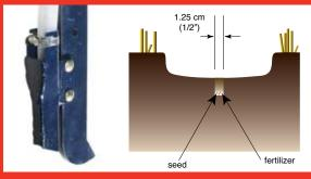
The **narrow knife single shoot opener** is a single shoot opener that places a narrow 1.25 cm (1/2") ribbon of seed in each seed row. This opener cuts a smooth narrow channel for seed to be placed, and has the lowest soil disturbance of the openers available on the Morris Contour Drill. This opener has proven to be a popular choice with growers with sticky, high clay content soils.
