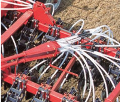
Morris' patented Flat Fan Divider Heads provide an accurate and efficient air delivery system that is exceptionally gentle on seed.
