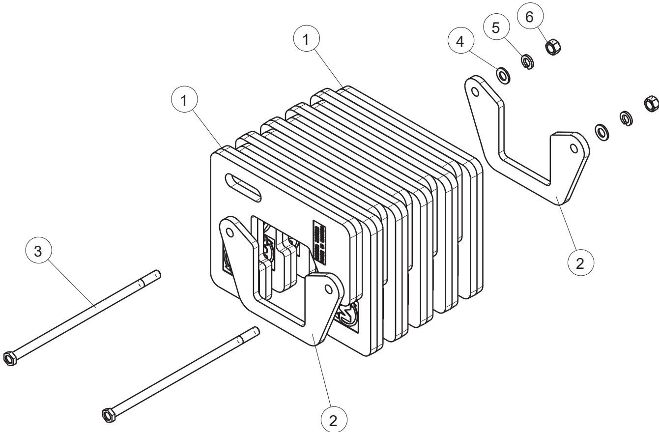
**Note: Wrap Wieghts (1) around beam alternating left to right.
