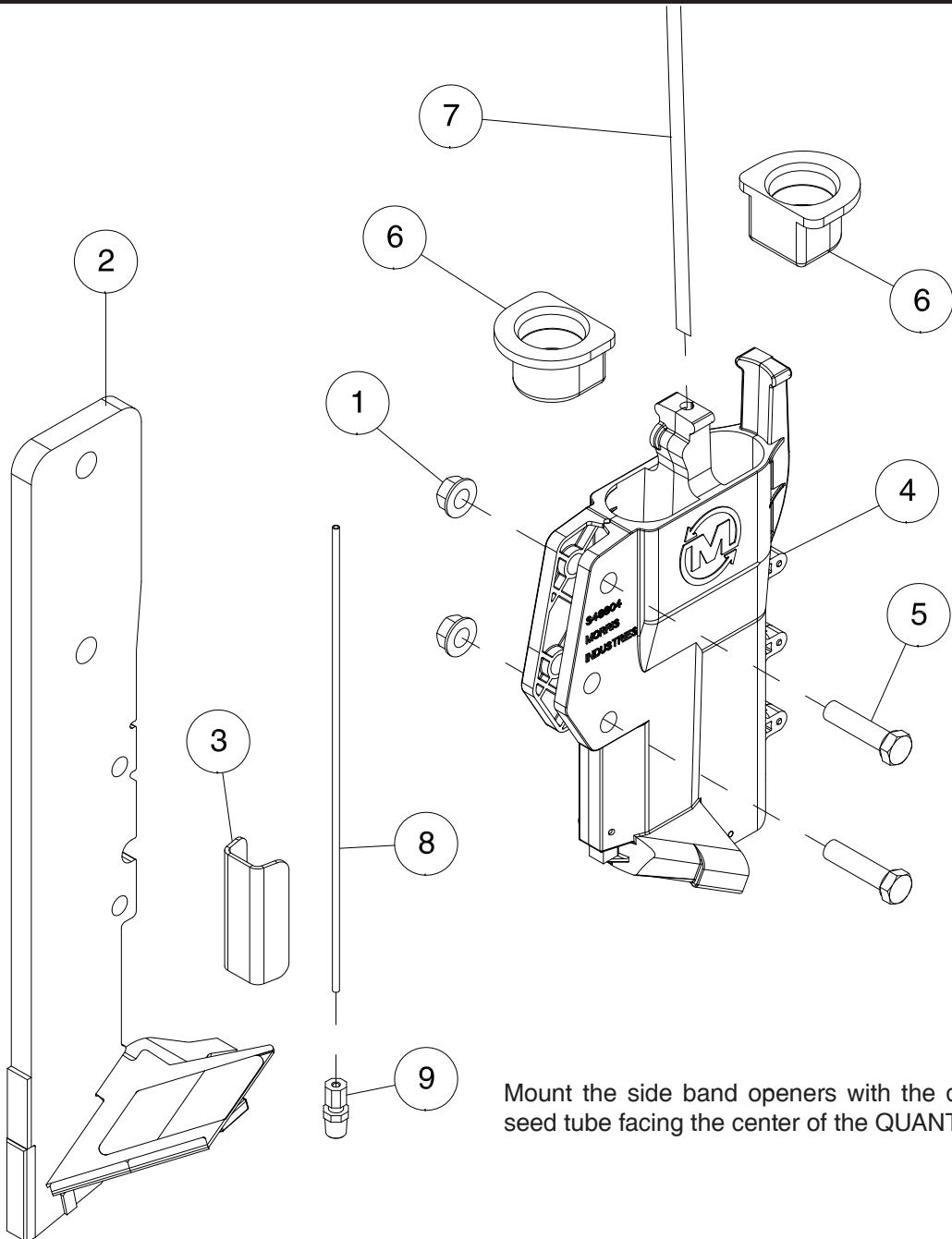
Mount the side band openers with the deflector and seed tube facing the center of the QUANTUM Air Drill.
