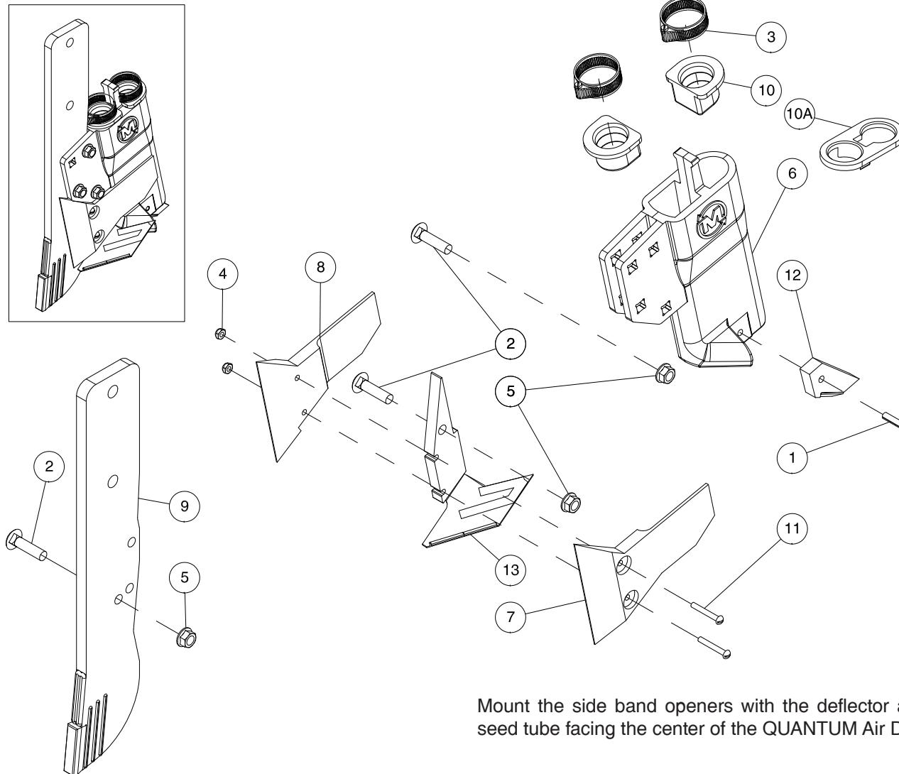
Mount the side band openers with the deflector and seed tube facing the center of the QUANTUM Air Drill.
