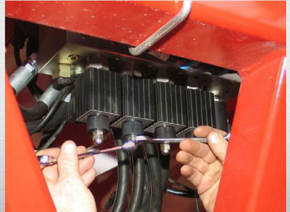
Remove Cap Nut and Loosen Jam Nut
