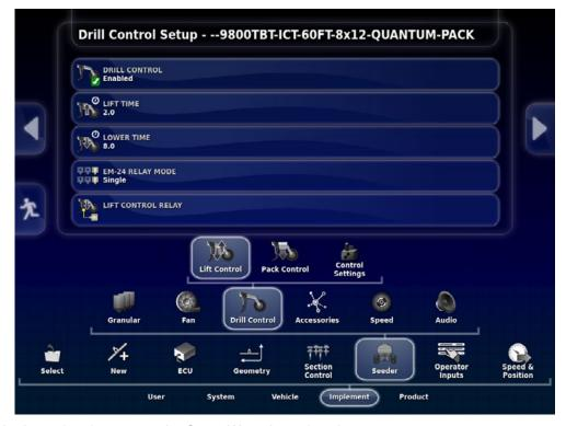
13.To adjust the Lowering time, press the Setup Wrench, and navigate to:
