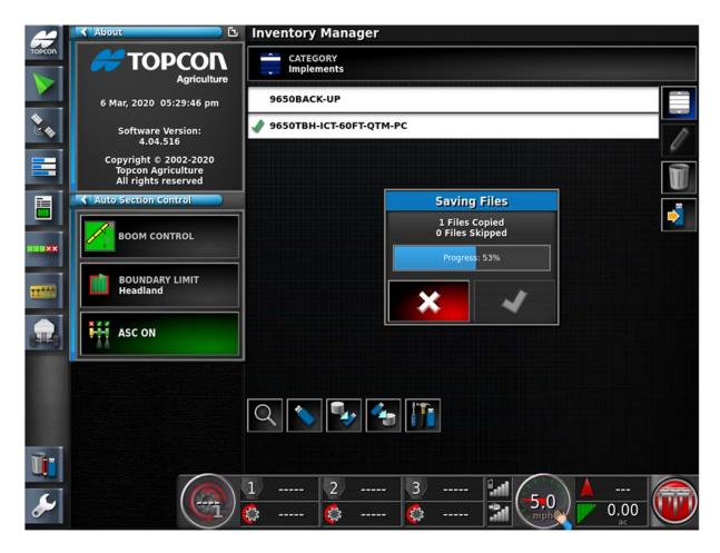
23. The backup profiles will be transferred to the USB stick. When Complete press the Green check mark and eject the USB stick by using the eject feature. With a label maker add the decal - Morris Back up profile. Keep this USB stick in a safe location.
