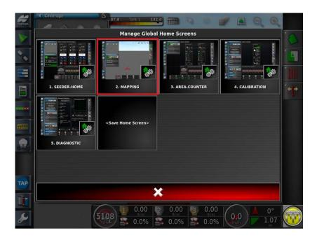
9. Press on the middle of Mapping Icon (do not press the small Gears Icon).
