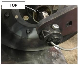
Pack Control Spindle Orientation - Top Decal Must be facing up.
