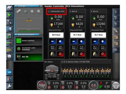
16. Press the top band to Minimize Tank 1
