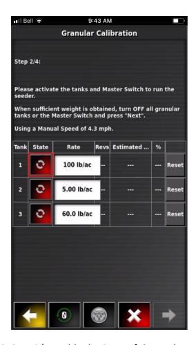
18. Step 2/4 Enable the State of the Tank you would like to Calibrate.
