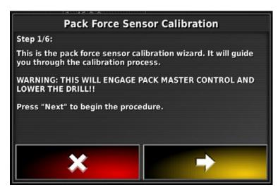
6. Read the Warning and check for bystanders once clear, engage the Tractor Lift Lower Hydraulics circuit - Followed by the Yellow arrow.
