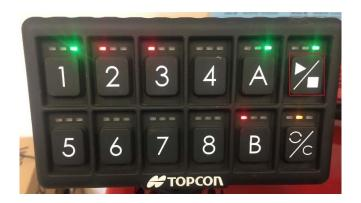
20. Turn the metering system ON by pressing the Start Key
