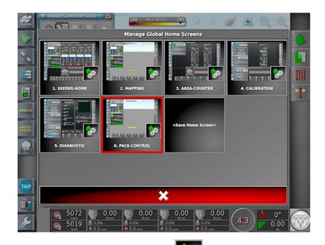
22.Swipe Up to reveal the dashboard ribbon and press the dashboard ribbon and press the center of the Pack-Control icon. Do not press the green house.
