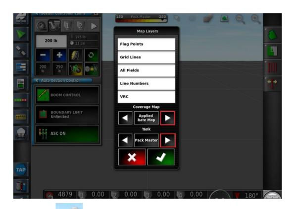
2. Open the **Map Layer** Icon, and toggle the Coverage Map arrow to **Applied Rate Map**, and the Tank Arrow to **Pack Control**. Apply the settings with the Green check mark.
