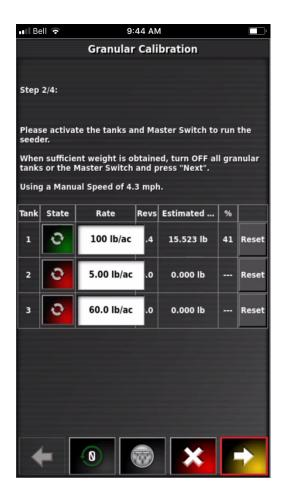
25. The Estimated Weight will count continuously as product is collected into the Sample Collector.
