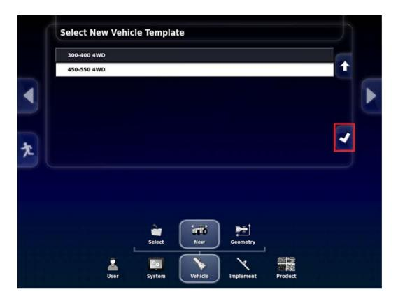
10. Select the Model of tractor from the list. Press the White Check mark to Continue.
