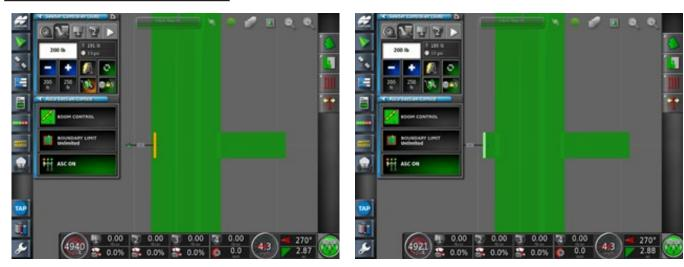
12.As the implement exits the previously treated area and passes into the untreated coverage area, the control system will automatically lower the implement.
