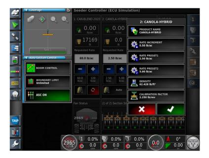
20. Adjust Increment settings, Rate presets and ensure a calibration value is entered, Review and proceed with the Green Check Mark.
