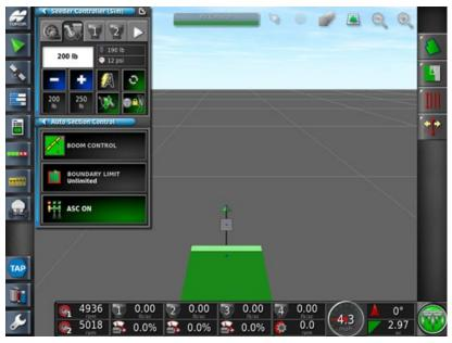
9. Continue to drive forward and create 3 back to back coverage passes. Drive approximately 2 squares on the map (650' / 200M). It is recommended to set an A/B line on the tractors steering system at this time.
