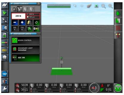
8. The Hydraulic Pressure will fluctuate depending on the soil conditions, this is normal as the control system is adjusting the hydraulic pressure continuously maintain the desired packing force over the variable field terrain.
