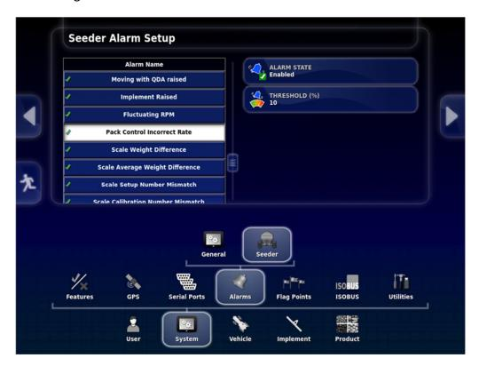
Pack Control Incorrect Rate - Threshold 10%
