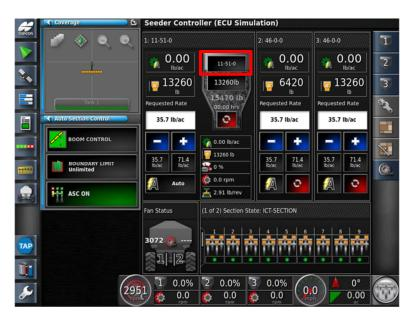
2. Press on the Top area of the Tank- to open the Product Configuration Window
