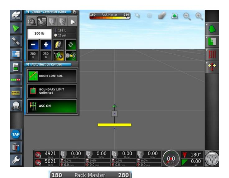
21.Note the legend now shows the Minimum and Maximum Pack force Values assigned. These colours will be displayed on the coverage map of the actual packing force applied in the field.
