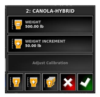
24. Using the keypad enter the **Weight manually.** Proceed by pressing the Green Check mark.
