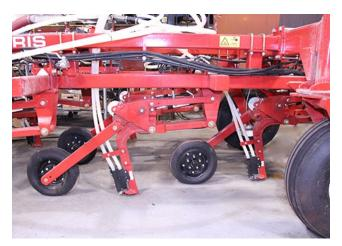
6. The openers will now begin to lower into the working position under hydraulic pressure.
