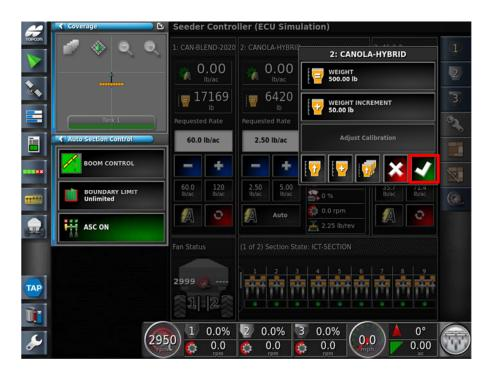
27. The tank weight is now **500lbs**. Apply the changes with the Green Check mark.
