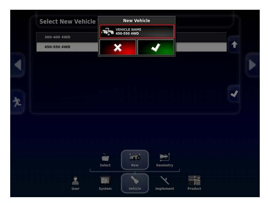
11. Adjust the name to match your model of tractor. Press on **Vehicle Name** Icon.
