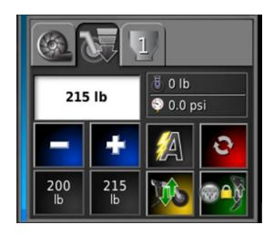
Special operation - Pack Control - On/Off (Float mode) button when toggled to OFF, allows the openers to Float over terrain in the downward working position with no pressure applied. This function is useful when travelling over a wash out or in muddy conditions when the unit is on the verge of becoming stuck. Using Float feature allows for the application of product to be broadcast on top of the ground.
