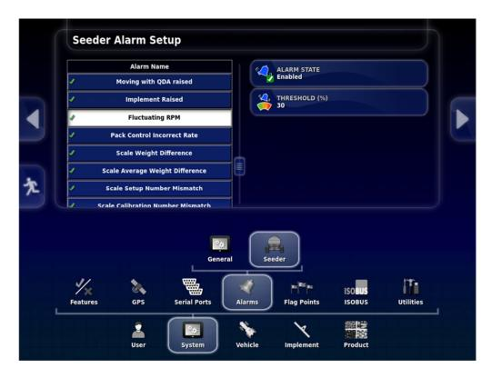
Fluctuating RPM - Threshold 30%
