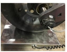
Note: The Loadcell decal Top must be facing Upwards.
