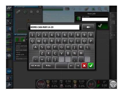
6. It is recommended to edit job name to match the current **Field and Date and Product** used. Example: **HOME-CAN-MAY-14-20**; apply the settings with the Green Check mark.
