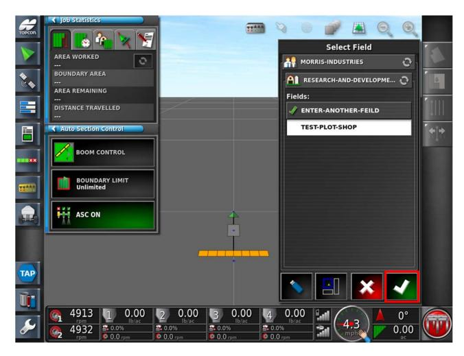
20. The fields we created are in the list. Notice how the last field we created has the Green Check beside it. Select the Field you wish to seed first. Press the Green Check mark to apply the settings.
