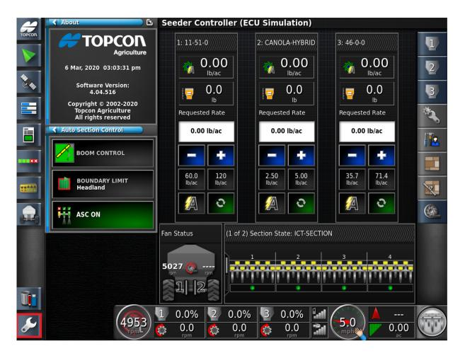
4. Press the Wrench on the Bottom Left Corner to enter the Set up Menu
