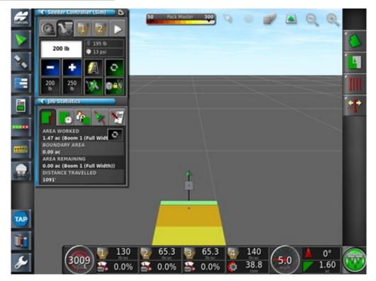
26. Since the system is now being commanded to apply 250lb of packing force, the pack control coverage map is now painting a different shade of colour. This is a quick reference and provides validation that the system is functioning correctly.
