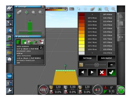
7. Press the **Auto Applied** icon followed by the Green Check mark. Repeat the above procedure on the remaining tanks.
