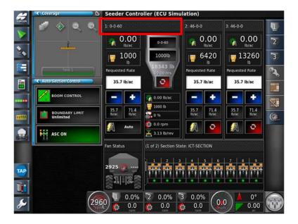
3. Expand the Tank you wish to add the Product into by pressing on the top Band.
