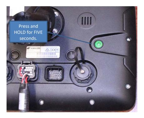
1. Press and hold the **Green Power** button, located on the back.
