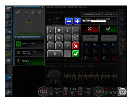
11. Using the keypad enter the following Cal factor 2.25 lb/Rev
