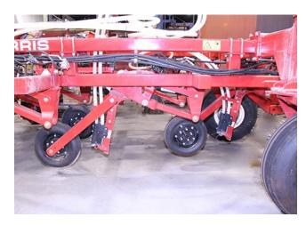
• Using the above settings, the Openers are being commanded from the Monitor to be in raised position.
