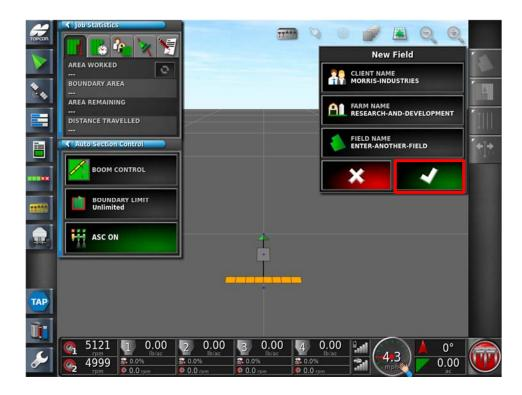
18. Apply the new Field Name with the Green Check mark. The field has now been saved. Repeat the above procedure to add all of your remaining fields into the X35's memory. Note: Remember to press the Green Check mark to Save the field name.
