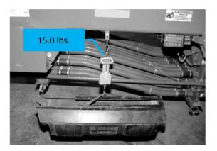
26. Remove the Collector Tray and Weigh the Product using the provided scale.
