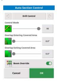
8. Adjust the Auto Section Control Threshold for ICT-Section 95% and Drill Control to 95%.
