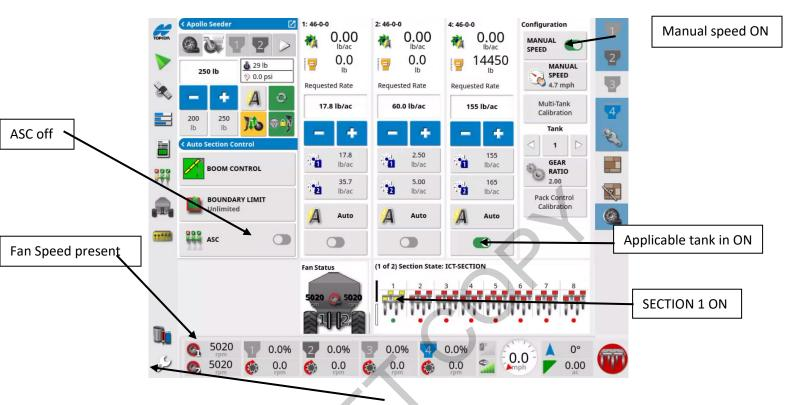
Sections can be turned on and off by touching the **Wrench**, then **Implement--Apollo seeder--Section control--Section switch**. Choose to enable or disable.
