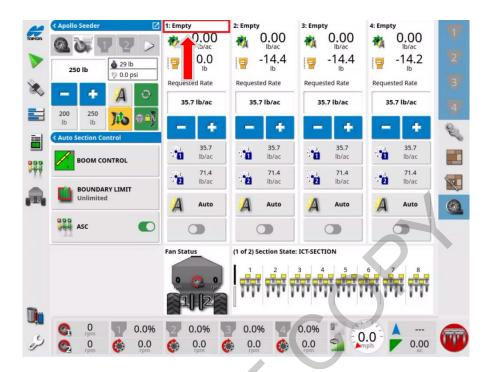
Press on the Top box of the Tank image to open the Product Configuration Window
