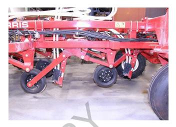
• Using the above settings, the Openers are being commanded from the Monitor to be in raised position.
