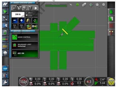
16. Notice how the entire implement must fully travel through the previously treated area, only once the entire drill is inside the coverage will the Lift command be activated.
