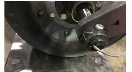
Note: The Loadcell decal Top must be facing Upwards.
