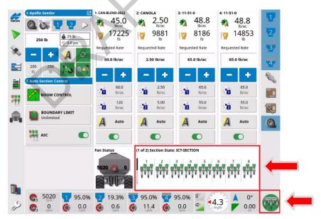
Note: There is a several second delay for features on the screen to change to the colour green, this is based on the transition time of the product from the metering wheels to the openers.
