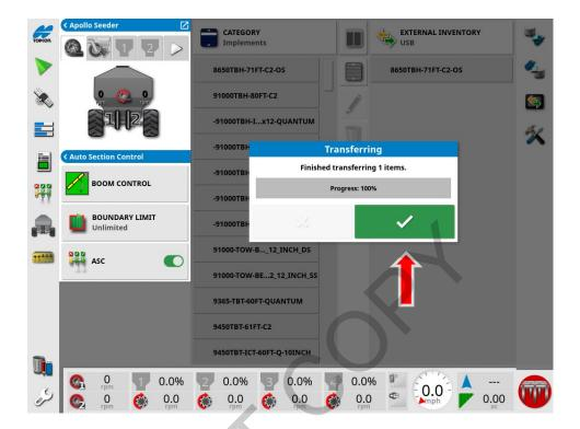
When Complete press the **Green check mark** and eject the USB stick by using the eject feature.
