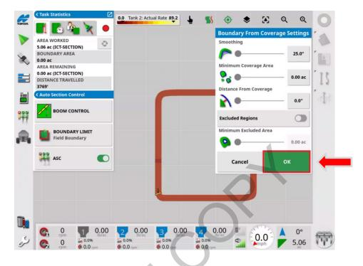
**Creating Boundaries** message will be displayed. The outer area of the boundary will darken with less visible grid lines. Accept the Boundary by proceeding with the Green check mark.
