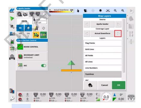
6. Open the **Map Layer** Icon, and Adjust the **Coverage Map** arrow to **Coverage** and the **Tank** arrow to **Pack Control**. Apply the settings with the Green check mark.
