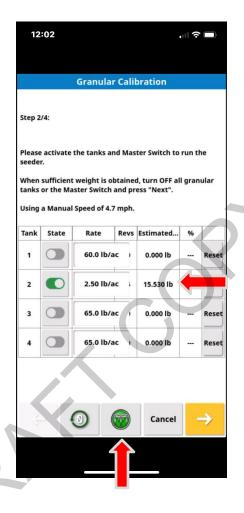
Stop the Metering when the Estimated weight is around <u>15.00lbs</u>. Proceed
