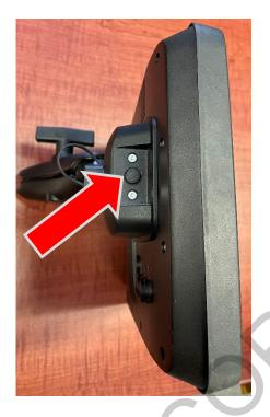
Press the power button, located on the left side of the unit.
