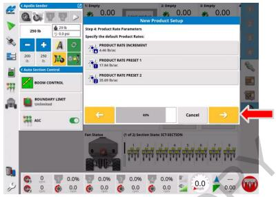
Rate increment- Used for quickly bumping the rates up or down (+/-) while moving.
