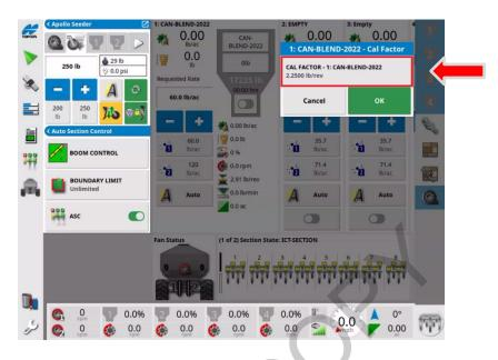
Using the keypad enter the following Cal factor 2.25 lb/Rev. Touch Green Check mark.
