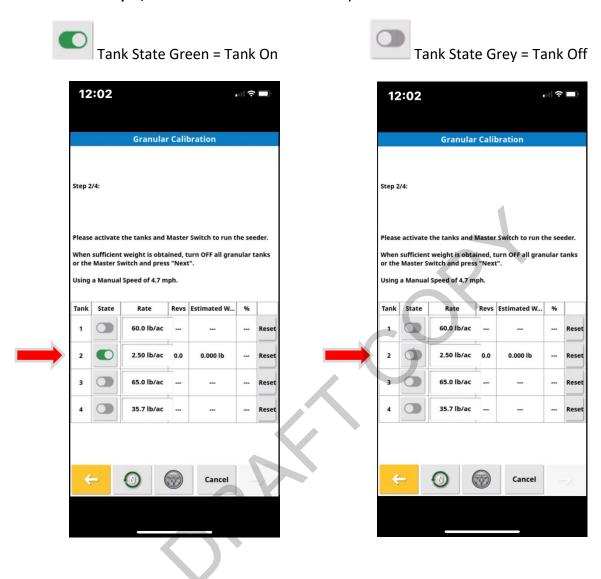
Metering is Active and is ready to discharge product. The Tank Preset 1 Rate will automatically be displayed.
