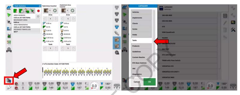
Once into the tasks tab, move through your client tree and select whichever field and resulting task you want. In this case it's the **MANUAL-TEST-TIMING** task.
