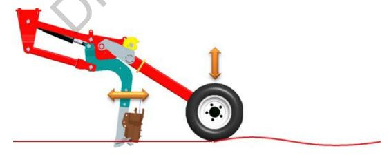
27. During a test pass, have someone drive along side the Quantum and inspect the openers. Communicate with each other on the current settings used and if the openers appear to be locked into the working position. If they
