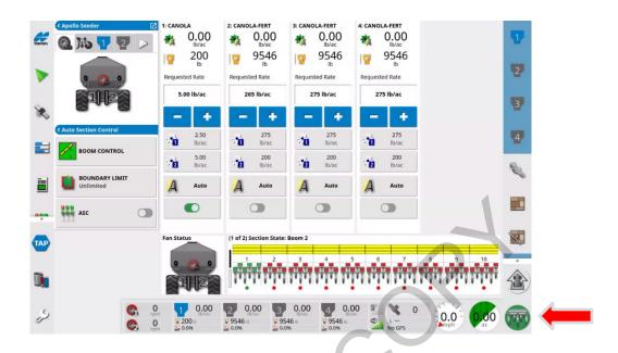
Product should have run out the bottom of the collector belonging to the selected tank. Once you have verified the product has been dispensed, turn off section 1, turn on section 2 and repeat for the remaining sections in tank 1.
