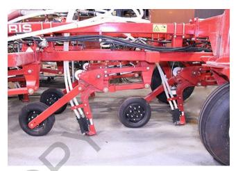
6. The openers will now begin to lower into the working position under hydraulic pressure.
