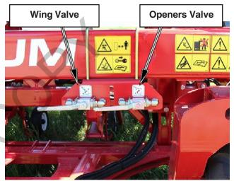
**Valves in Unlocked Position**
