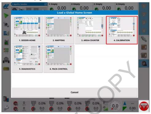
Perform a calibration of the test product for each tank. Refer to the calibration section of the X35 User Guide if needed.
