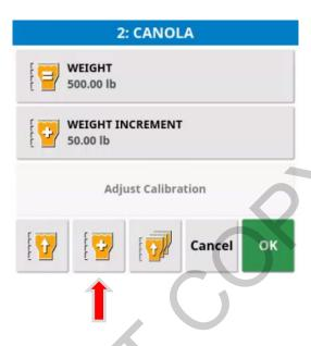
The tank weight is now **500lbs**. Apply the changes with the Green Check mark.
