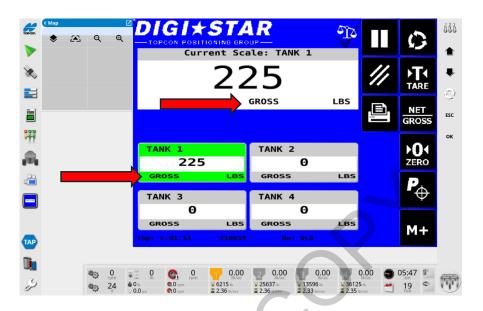
• With the desired tank selected, select the "tare" button to set the "Net" value of product in the tank to 0.
