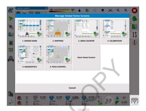
21. Swipe Up to reveal the dashboard ribbon and press the center of the Pack-Control icon. Do not press the green house.
