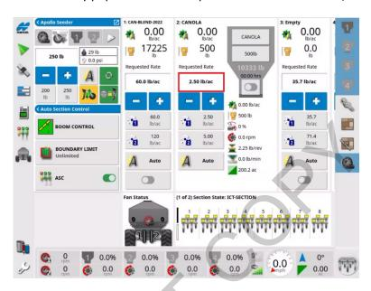
Continue to add products into the Tanks 3 or 4 by touching the top band for desired tank and repeat
