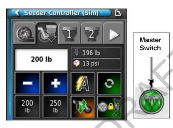
Pressing the Master switch, the openers will now begin to lower into the working position. Cycle the openers several times up and down to ensure proper functionality.
