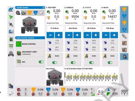
Navigate to **IMPLEMENT—APOLLO SEEDER—SECTION CONTROL—TIMING.** Adjust the section ON/OFF times based on your documented times. Simply touch the applicable section and input the desired time.
