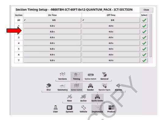
Adjustments can be made to achieve a safe level of overlap. Simply touch on the section you wish to fine tune, and enter a new time, and accept with the green check mark.
