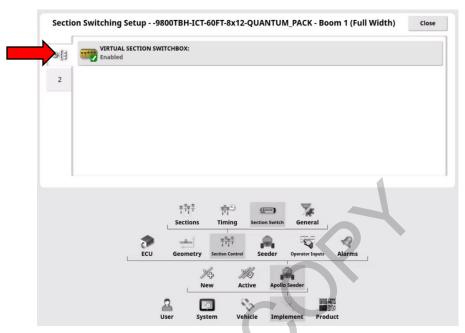
The section switch should only be used during the setup procedure. The switchbox can cause sections to be turned off accidentally by careless operator error.
