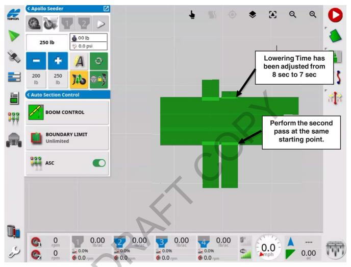
14. Drive around and make a second pass starting at the same side as the first pass, this will make it easier to compare the Lift and lower times against each other.
