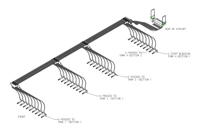
9. Start at the rear of the aircart (Tank 4 - Section 1 hydraulic cylinder). This method applies to both TBT and TBW aircarts. Follow the above diagram.
