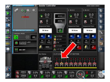
19. Turn OFF Section #1, Turn ON Section #2. Repeat the above procedure on the remaining sections.
