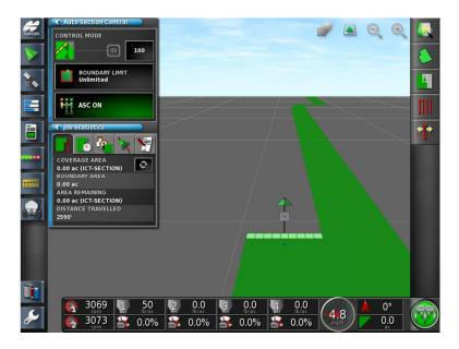
8. First make two back to back passes covering roughly 300m in each direction. This will create two swath widths of coverage area. It is recommended to set an A-B line on your guidance system to avoid any gaps. It is recommended to only "scratch" the surface of the soil during these first two passes.
