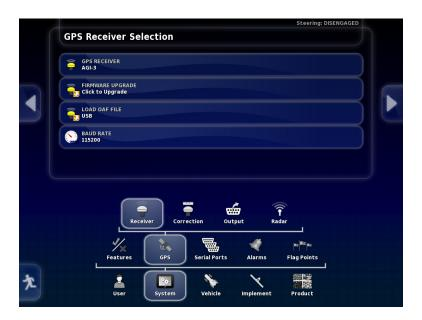
9. Change the Receiver type to AGI-3, with Baud Rate of 115200.
