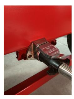
3. Connect the **Morris handheld Switch box** power harness to the **Trailer Plug receptacle** on the back of the Aircart.
