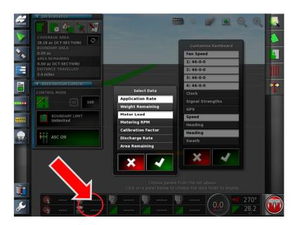
28. Customize the **Dash Board** by simply tapping on the bottom row of icons. Adjust the **Select Data** to include: **Application Rate** and **Motor Load.** Apply your changes with the Green checkmark.
