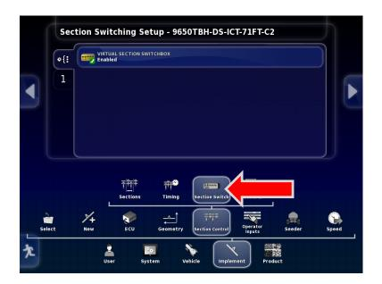
23. Navigate to - Implement - Section control - Section Switch
