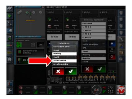
13. Ensure **Heading** and **Area Covered** is highlighted. Apply with the Green Check mark on both Menus.
