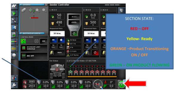
TIP: WATCHING THE MOTOR LOAD / PWM VALVE IS A GOOD REFERENCE TO LET YOU KNOW THE MOTOR HAS ENGAGED.
