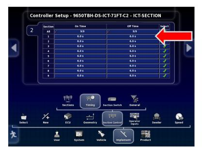
22. Navigate to – **Implement - Section control – Timing.** Adjust the Section ON / OFF Times based on your collected data.
