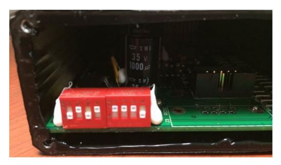
3. Monitor ECU – check to ensure the Dip switches are set correctly. Note: the location of the capacitor for reference.
