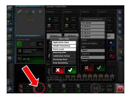
9. While the **Customize Dashboard** option is open, by tapping the Dashboard again within the **Tank 1 Zone** will allow for further customization. Notice how the **Select Data** window is now visible.
