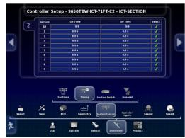
1. The monitor Section Timing will automatically turn the metering system ON several seconds ahead to compensate for the lag time it take to product to travel through the airstream to the openers.
