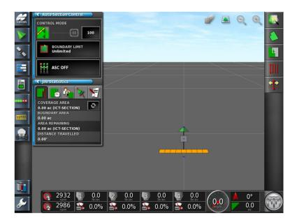
2. Drive your tractor and implement into an open field. You will need a fairly large open area as we will be making several large passes in each direction to "Dial-in" our Section ON/OFF times.
