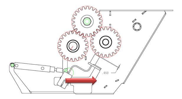
13. Review the error codes and adjust the required section sensors which are located in-between the metering bodies. Adjust the Gap to .031" - .064"
