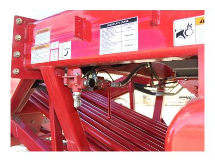
2. Aircart hydraulic flow Knob is **OUT** for **FAN**, move lever to **CALIBRATE**.
