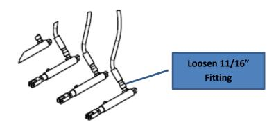
10. Place collection bucket underneath the cylinder. Hold the elbow fitting (on the cylinder) firmly with your 7/16" wrench, use the 11/16" wrench to break loose the hydraulic hose fitting.
