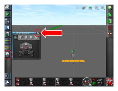
1. The **Seeder Controller** must be fully expanded. Hide any of the mini windows by pressing the small **Left Arrows**.
