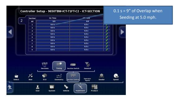
15. Adjust the Section timing to a safe level of overlap.
