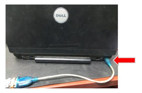
1. Turn on Laptop Ensure the USB to Serial adapter is plugged into the Rear USB port. It may take several minutes for the Prolific Device drivers to self-install.
