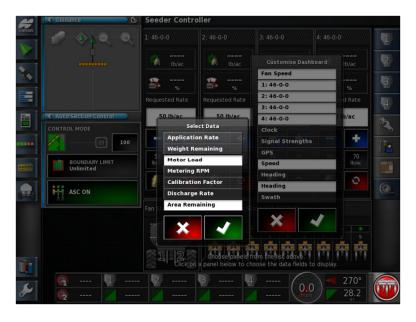
10. Adjust the **Select Data** to include: **Motor Load,** and **Area Remaining.** Apply your changes with the Green check mark.
