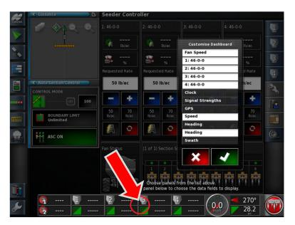
8. Customize the Dash Board by simply tapping on the bottom row of icons. ENABLE THE FOLLOWING:
