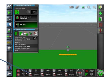
TIP: WATCHING THE MOTOR LOAD GAUGE WILL ALLOW YOU TO KNOW WHEN THE METERING HAS ENGAGED / DISENGAGED
