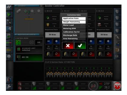
15. Adjust Tank information to include Application Rate and Weight Remaining.
