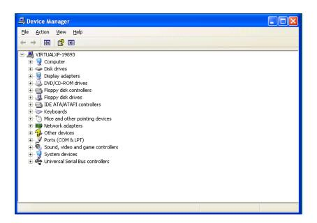
6. Expand Ports (COM & LPT) by pressing on the + symbol.
