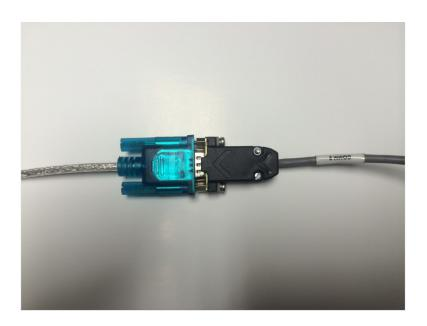
2. Connect the USB 9 pin to the COMM 2 Input on the AGA5072 Harness.
