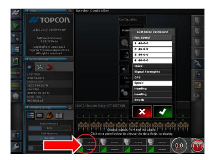
45. While the **Customize Dashboard** option is open, by tapping the Dashboard again within the **Tank 1 Zone** will allow for further customization.
