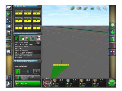
16. With the timing dialed in experiment with the ICT system. You can now seeding on a 45° angle. Experiment with the Overlap Control to which best suit your conditions.
