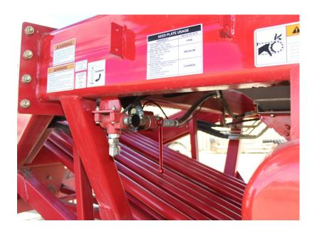
10. Once the Calibrations are completed. DIVERT THE OIL FLOW BACK TO THE FAN!!! CLOSE THE LIDS AND RESUME THE AIRCART FOR NORMAL SEEDING OPERATION (PRODUCT DIVERTERS).
