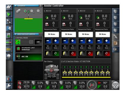
3. Turn **ON** the Tank which is the furthest away from the drill.
