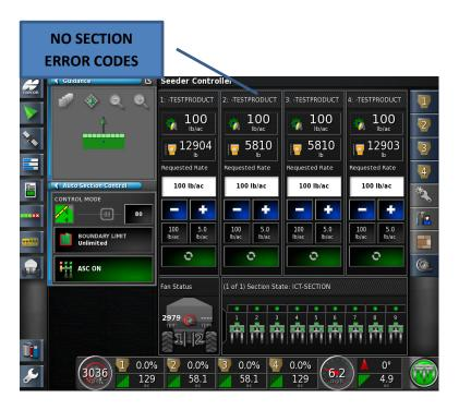
14. Run the system again, repeat procedure until no errors codes are present.
