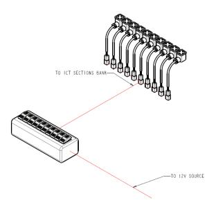
4. Connect the Morris handheld switchbox granular section harness to the 1-9 Pigtail adapters on the back of the aircart. You may need to temporally disconnect the factory installed harness.
