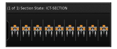
6. Orange = Product is transitioning On/OFF between Metering and Openers.
