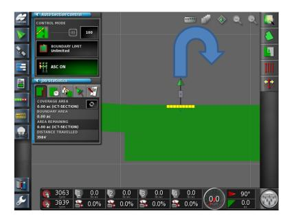
10. Drive forward 100 yards and then make a U-turn and head into the covered area at normal operating speed.
