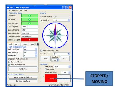
7. On the laptop press the Stopped icon, it will change green and show moving. The Speed will be displayed on the X30 monitor.
