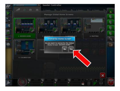
51. If you ever need to make adjustments to the screen templates, example (Adjusting Map layers) the screens layouts must be **resaved** after any changes have been made. To save the changes just hold the **Topcon logo for 5 seconds** and select the icon of the screen you modified. Tap **yes** to use **the Overwrite Home Screen** feature.
