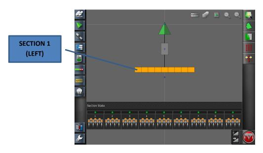
16. SECTION 1 is ALWAYS the outer LEFT WING (DIAGRAM IS FOR REFERENCE ONLY).
