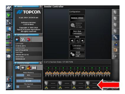
47. Continue adding **Calibration Factor** and **Motor Load** the remaining **Tanks Zones**. Apply with the Green Checkmark.
