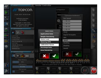
46. Highlight only **Calibration Factor** and **Motor Load**. Apply with the Green checkmark.
