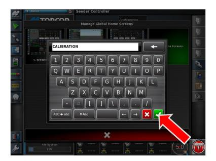
49. Name this Layout: **CALIBRATION.** Apply the settings by pressing the **Green Check mark**.
