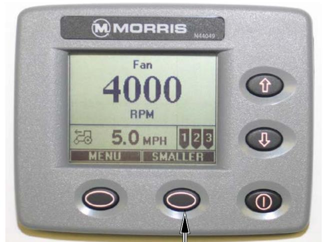
Pressing soft key under SMALLER will switch the screen back to the two - display sections.
