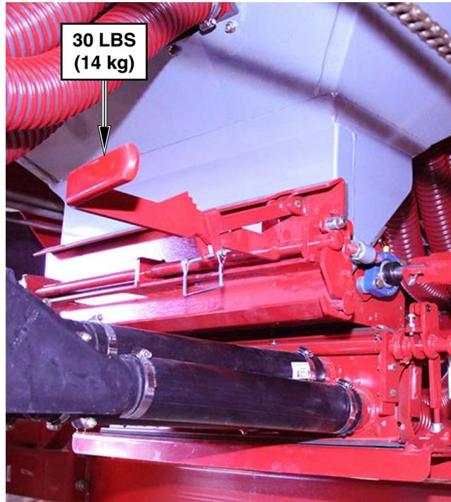
**Adjust the latch bolts to obtain a force of 25 lbs to 30 lbs (12-14 kg) to close the Door.**
