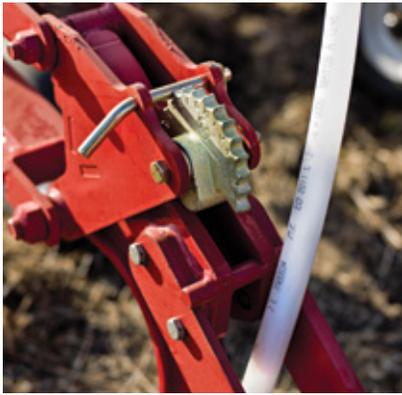
The one-to-one parallel linkage maintains a constant opener angle relative to the soil and opener depth relative to the packer wheel throughout its range of travel. The opener can contour up 25 cm (10 inches) and down 18 cm (7 inches).
