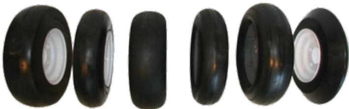
Packer wheel options: 5.50" x 16" Semi-Pneumatic, 4.80" x 16" Pneumatic, 4.80" x 16" Semi-Pneumatic, 4.50" x 16" Semi-Pneumatic Otico tire, 5.50" x 16" Semi-Pneumatic Otico tire and 4.00" x 16" "V" Crown.
